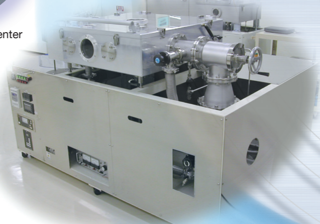
Test rig for bearings for vacuum conditions
